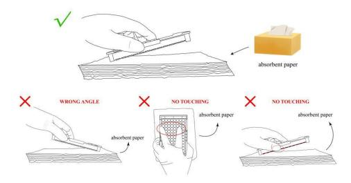
i) Schematic diagram of tapping the plate:
